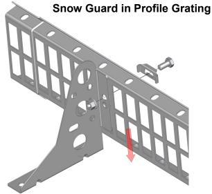
The profile grating is assembled on the mount using M10 bolt + nut + clamp. Max. overhang 300 mm. Adjust the grating downwards against the roof for less gap.
