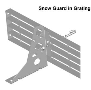
The grating is assembled on the mount using J -hook M8 + nut. Max. overhang 300 mm.
