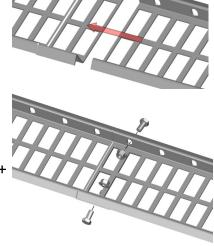
The **Ice Guard** is pushed together and mounted using fishplate brackets and 4 M10x20 bolts + nuts.
