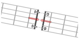
The **Grating** is pushed together and screwed in place using 2 M10 bolts + nuts
