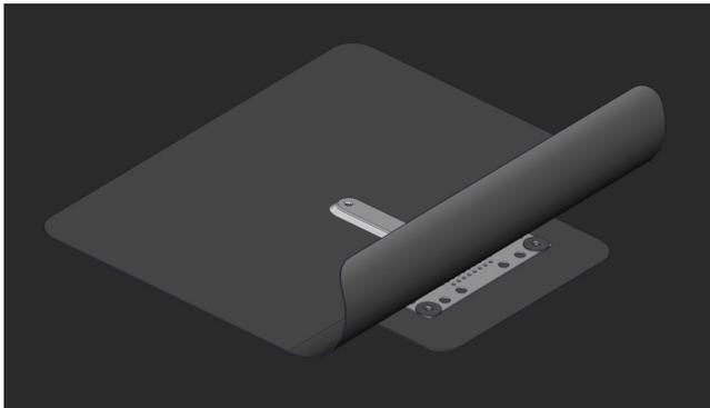
When assembling spacers for ladder or gangway, the sealing plate is rotated by 90 degrees.
