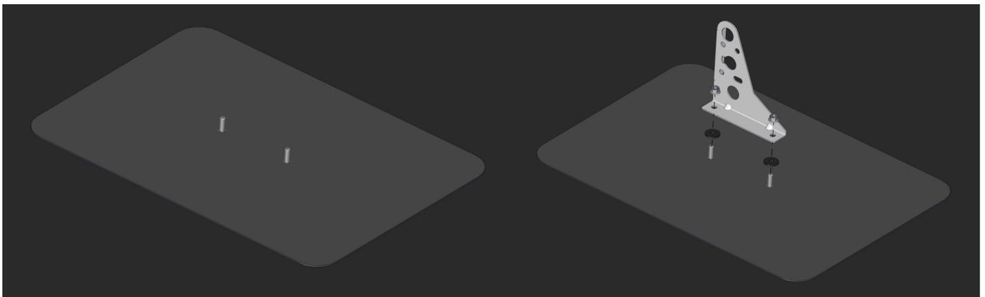
Cut out a repair patch with holes for the mounting bolt. The plate should have a min. thickness of 1.2mm and cover at least 50mm around the sealing plate.
