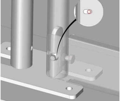
The kick strip is mounted using 2 self-drilling screws.
