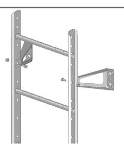
Assemble the ladder in the top pair of brackets using 2x M10x20 + nut and make sure the top rung is at least 30 mm above the roof edge.
