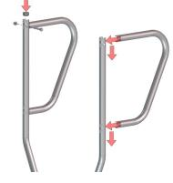
Assemble any handrail and hoops The hoops are hooked and knocked into the track, lock with M10x60 bolt + nut.
