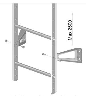
Install the remaining brackets with max. c/c distance of 2500 mm.
