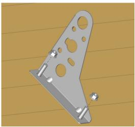
Screw the bracket into place using 2 M10 nuts.
