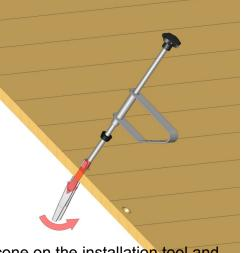
Thread the rubber cone on the installation tool and screw on the quick fixing mount. Then push the quick fixing mount into the hole and make sure the arm opens out.
