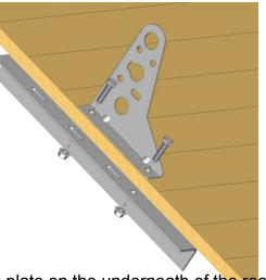
Place the backing plate on the underneath of the roof and the bracket on the top, Screw into place with 2 M10x60 mm + rubber washer and nuts.
