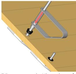
Pull the arm up against the under-roof and push the rubber cone firmly into the hole. Unscrew the installation tool. **NOTE! The mark in the bolt must be perpendicular to the direction of the boards.**
