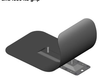
Place a repair patch on top and fuse together. Alternatively, use "Icopal roofing adhesive" or other suitable sealing compound.
