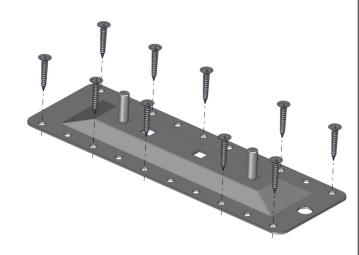
Place 2 M10 coach bolts into the outer holes of the base plate before you screw it into place using 10 6x35 wood screws. **Use a screwdriver with a deep stopper base so the screw doesn't go round and lose its grip**
